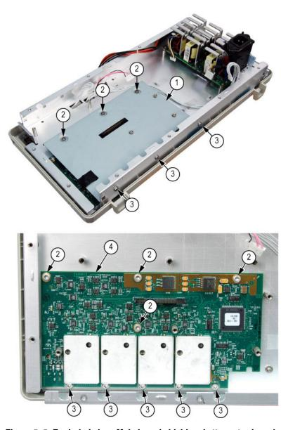
Figure 5-5: Exploded view: Main board shield and attenuator board
