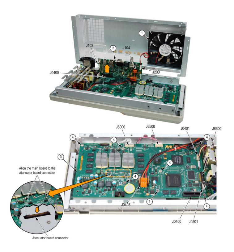
Figure 5-2: Exploded view: DPO3000 I/O and main boards
