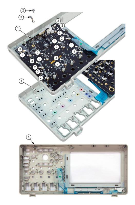
Figure 5-7: Exploded view: DPO3000 front panel board and front case
