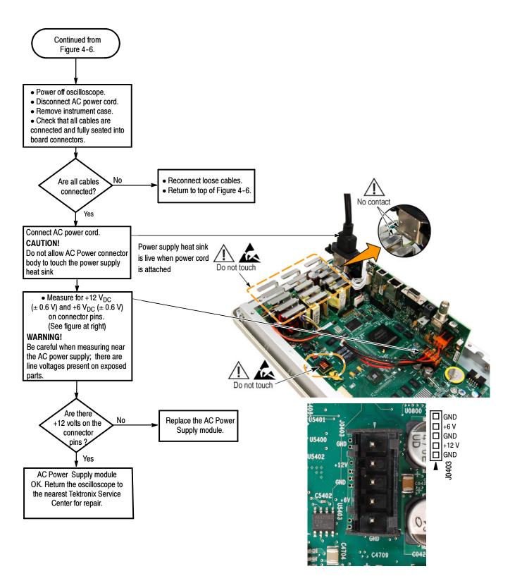
Figure 4-7: AC power supply troubleshooting procedure
