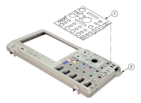
Figure 5-4: Exploded view: DPO3000 front panel labels
