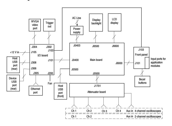
Figure 2-1: Oscilloscope module interconnections
