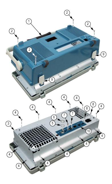
Figure 5-1: Exploded view, rear case and rear chassis
