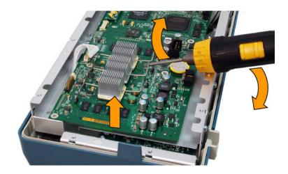
Figure 4-4: Disconnecting the Main board
