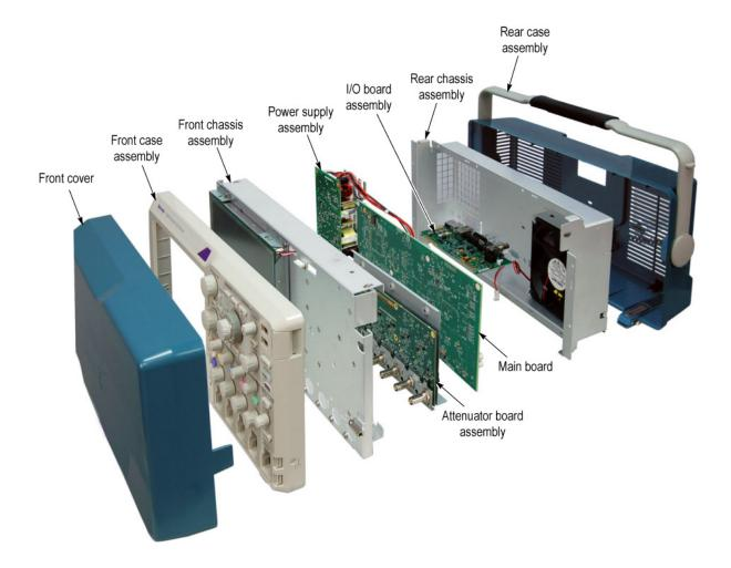
Figure 4-1: Locator for internal modules
