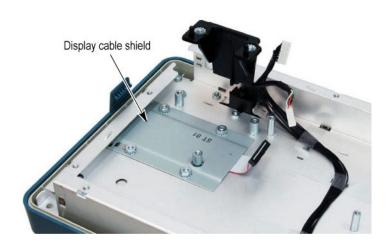
Figure 4-5: Display cable shield in place
