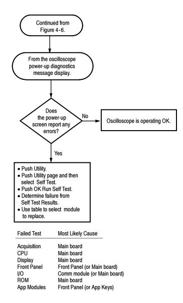
Figure 4-8: Module isolation troubleshooting procedure
