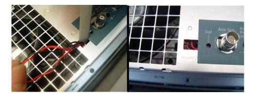
Figure 4-2: Reconnecting the fan cable
